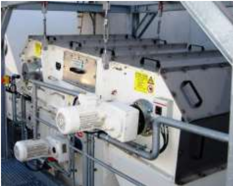
Image 4: A powerful magnet above the conveyor pulls ferrous metals like screws and nails out of the mass.
