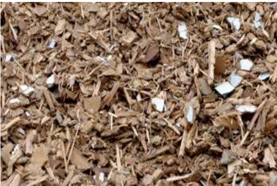
Image 2: The boiler is fired with wood chips and waste wood and the biomass has to be processed accordingly.
